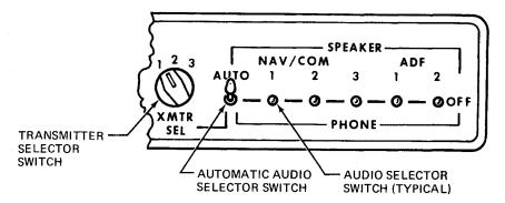
As illustrated, the number 1 transmitter is selected, the AUTO selector switch is in the SPEAKER position, and the NAV/COM 1, 2 and 3 and ADF 1 and 2 audio selector switches are in the OFF position. With the switches set as shown, the pilot will transmit on the number 1 transmitter and hear the number 1 NAV/COM receiver through the airplane speaker.
