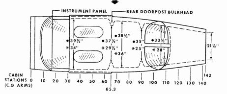
Figure 6-4. Internal Cabin Dimensions
