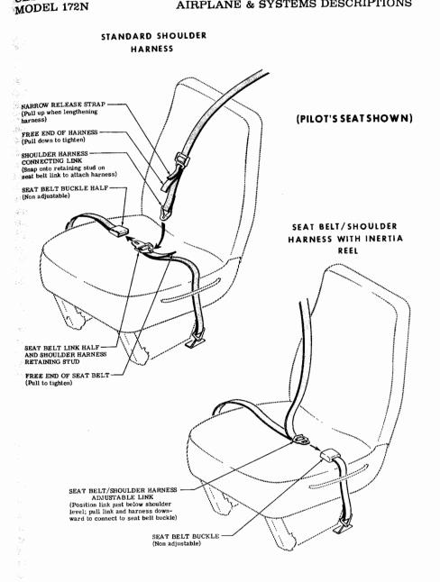
Figure 7-4. Seat Belts and Shoulder Harnesses
