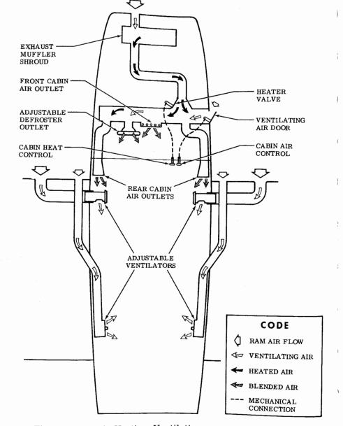
Figure 7-8. Cabin Heating, Ventilating, and Defrosting System
